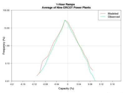
Figure 1. The 60-minute changes in power output during 2015 at nine ERCOT facilities (measured on a logarithmic scale).
