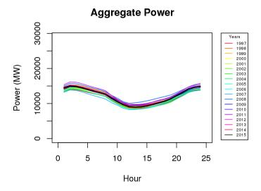
Figure 2. Average diurnal power profile for the years 1997-2015 using the WRF model (aggregate of all sites). Note that the profile for the year 2015 is highlighted in black.
