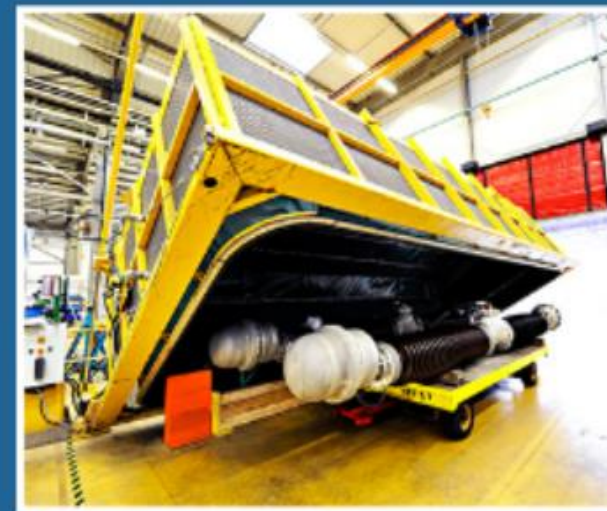
Circuit breakers are tested fully assembled for SF 6 gas tightness
