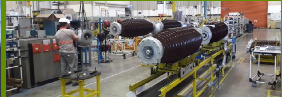
Circuit Breaker Assembly and testing
