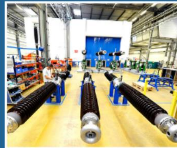
Live tank circuit breakers assembly complying with latest quality and EHS standards
