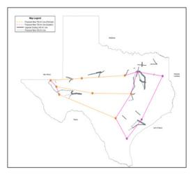
765-kV Core Plan with 345-kV New Lines and Upgrades Needed for the TX 765-kV STEP
