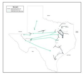
345-kV New Lines and Upgrades Needed with the 345-kV Plan
